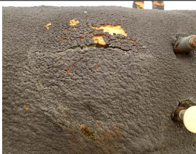
One of the locations on the vessel where the insulation is disbonding and blistering.
