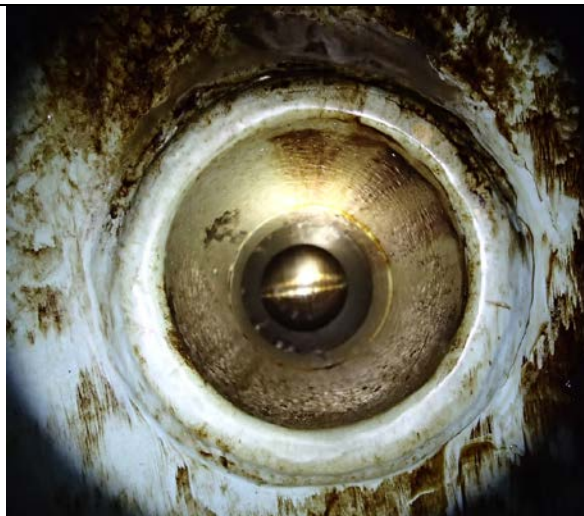
Inside the desand nozzle in the middle of the vessel.
